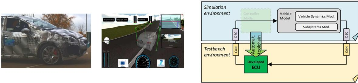
Fig. 1: Eunice MiW vehicle; Tecnia Dynacar simulator; MBD methodology [1, 6]
