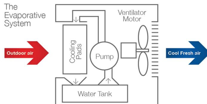
Fig. 1: Direct evaporative cooling working principle
