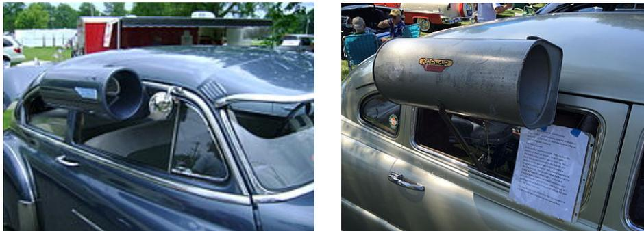
Fig. 2: Car coolers mounted on 1950s vehicles
